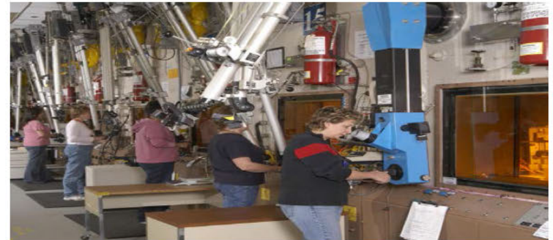
Shielded Cells in SRNL for High Rad Work
