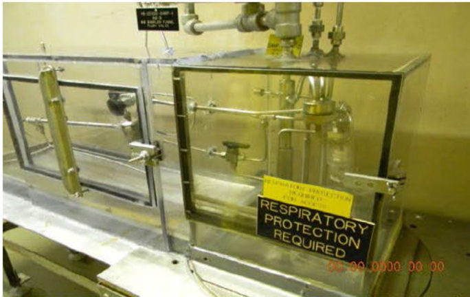
Sampler in H-Canyon (Long Path Ultra- Violet / Visible Light)
